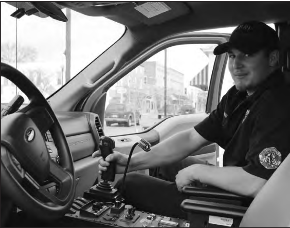
The Perry Fire Department's newest brush truck has "a bunch of gadgets," including a joystick-operated front-mounted hose. Above and below left, firefighter Chase Barineau demonstrates the device. Above right, Captain Elton Caraway shows off some of the equipment contained inside the truck, including generators, foam for chemical fires and axes.
