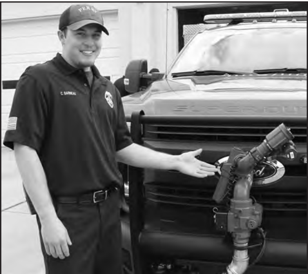
The Perry Fire Department's newest brush truck has "a bunch of gadgets," including a joystick-operated front-mounted hose. Above and below left, firefighter Chase Barineau demonstrates the device. Above right, Captain Elton Caraway shows off some of the equipment contained inside the truck, including generators, foam for chemical fires and axes.
